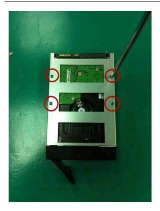
Once the HDD is placed in the tray, flip it over, align the tray screw holes with the HDD screw holes and secure the HDD with the supplied screws (Flat head  $#6-32 \times 4$ ).
